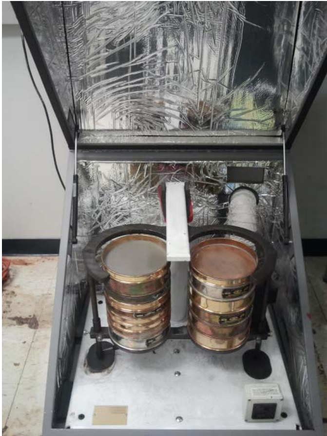
Shaker machine, implementing sieving mechanism to categorize particles
